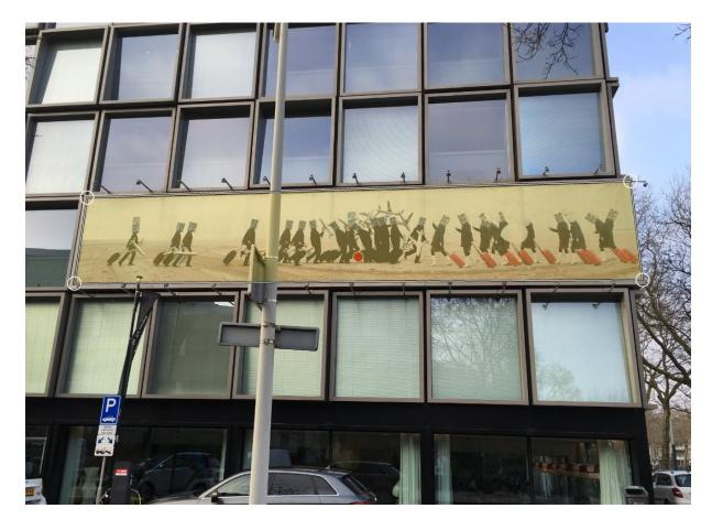
Since the sign is the object to be measured, the sign has been used for the alignment rectangle and the Spike laser (orange dot) is near the center of the alignment. Where possible the alignmen rectangle should encompass the area to be measured.
