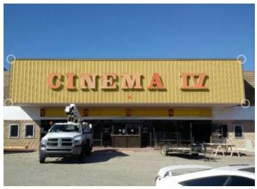
The whole area has been used in this example. Note the Spike laser is not on the raised letters but on the surface we are measuring. To measure the letters either measure them on the background surface beside the letters or aim the laser at the letters and use the top and bottom of the letters plus the two "I's" to create the sides
